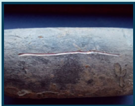
A lead pipe can be easily scratched with a key. (photo courtesy of US EPA Region 5)
